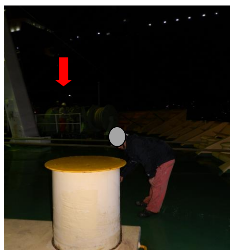
Figure 11: Approximate position of the A/B1 at the moment of the accident; in the background the position of the Bosun, controlling the winch, is indicated with a red arrow (photo taken during the simulation of the accident).
