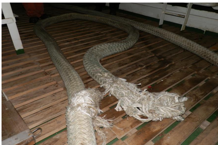
Figure 9: The spliced eye of the rope which the crew members tried to repair.
