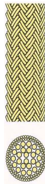
Figure 8 : Depiction of a standard double braided fibre rope:
